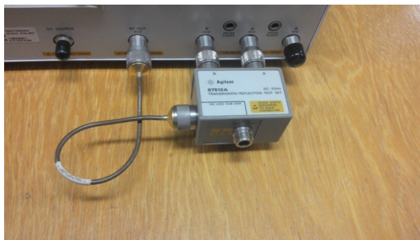
Figura 2. Transmissor/Reflector Agilent 87512A, ins loss 10 dB
